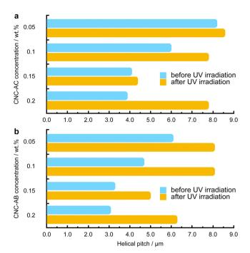
Fig. 4 Plots of the measured helical pitch (p) at 5 °C above the N-SmA phase transition on cooling from the isotropic liquid phase versus the concentration of (a) CNC-AC and (b) CNC-AB. Light blue upper data bars in each plot and for each concentration are samples prior to illumination with UV light and yellow lower bars after UV illumination.
