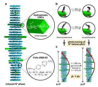
Fig. 2 (a) Schematic representation of the N\*-LC phase induced by the addition of minute amounts of the functionalized CNCs in the N-LC host, Felix-2300-03. (b) The trans-cis photoisomerization of the azobenzene pendants (AC or AB) induced by illumination with UV light (at  $\lambda=365$  nm) to prompt (c) an increase in the helical pitch (p) when the azobenzenes are in their cis configuration.
