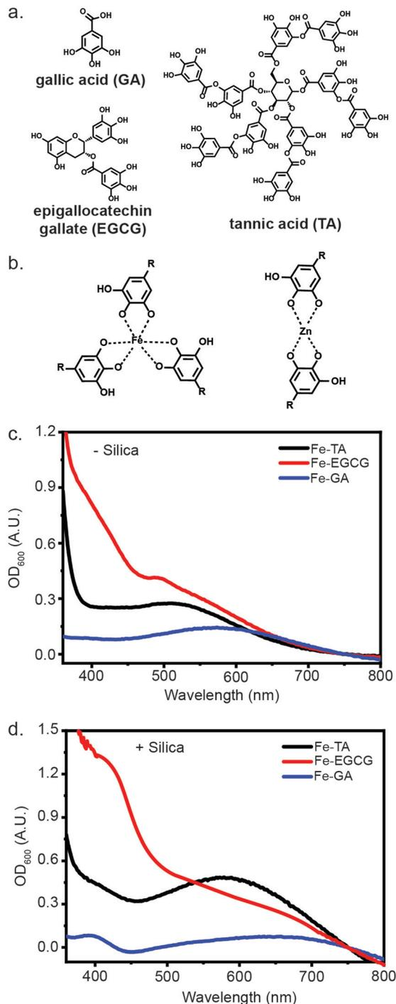
Fig. 1 Abiotic characterization of metal-phenolic networks (MPNs). (a) Polyphenol components used in the MPN assemblies. (b) Example chelation of metal ions (Fe<sup>III</sup> and Zn<sup>II</sup>) to polyphenols. (c) UV-Vis absorbance of Fe<sup>III</sup>-TA, Fe<sup>III</sup>-GA, and Fe<sup>III</sup>-EGCG complexes in MOPS buffer (10 mM, pH 7.5). (d) Fe<sup>III</sup>-TA, Fe<sup>III</sup>-GA, and Fe<sup>III</sup>-EGCG complexes formed on the surface of silica particles (1 mg mL<sup>-1</sup>).
