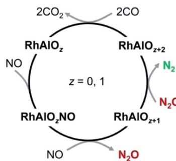
Scheme 1 Proposed catalytic cycle for the conversion of \text{NO} and \text{CO} into \text{N}_2 and \text{CO}_2 mediated by the neutral \text{RhAlO}_{0-3} species. This catalysis can also be driven by the \text{RhAl}_2\text{O}_{1-4} clusters.
