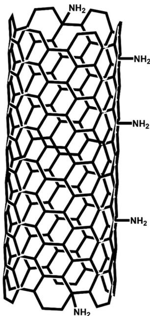
Fig. 9 Schematic structure of the single layer of MWCNTs-NH<sub>2</sub>.
