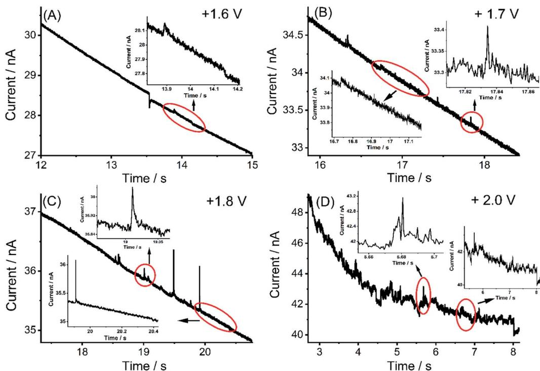
Fig. 3 (A)–(D) Examples of representative chronoamperometric profiles of nano-impact at different potentials (1.60, 1.70, 1.80 and 2.00) in a 0.1 M  $\text{KNO}_3$  (pH = 6.4) solution containing  $0.01 \text{ g L}^{-1}$  MWCNTs. No spikes or steps were detected below/at 1.50 V.
