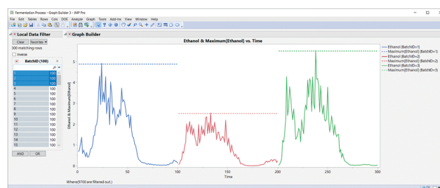
Fig. 19 Model inputs for batch processes can be generated by summarizing the information, which is known as landmark points in the literature. Here, the maximum temperature reached during fermentation can be found to be correlated to the quality of the batch.
