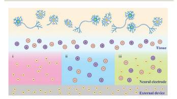
Fig. 4 Schematic diagram of the charge transfer mechanism of neural electrode materials: (i) charge transfer by electrons, (ii) charge transfer by ions, and (iii) charge transfer by the synergetic effect of electrons and
