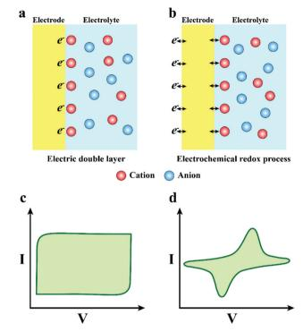
Fig. 3 (a) Schematic drawing of the capacitive charge injection mechanism (electric double layer), (b) Faraday charge injection mechanism (electrochemical process), and (c and d) their corresponding cyclic response.
