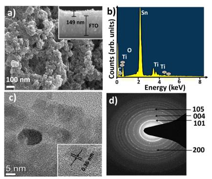
Fig. 3 (a) FESEM plan-view image, (b) EDX pattern, (c) HR-TEM image, and (d) SAED pattern of SILAR-grown TiO<sub>2</sub> film. Adapted with permission from ref. 23. Copyright (2018), Springer Nature Research.
