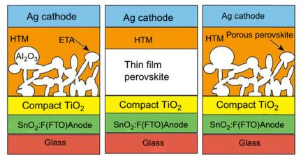
Fig. 6 Typical configuration structures of a PSC. Adapted with permission from ref. 47, Copyright (2018), Elsevier.
