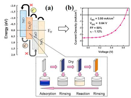
Fig. 5 The schematic energy level diagram and current–voltage characteristics of the NiO/Cu<sub>2</sub>O/ZnO/SnO<sub>2</sub> heterojunction flexible solar cell. Adapted with permission from ref. 42, Copyright (2016), Elsevier.
