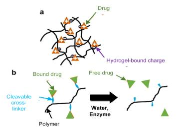
**Fig. 1** Drug-hydrogel interaction strategy, (a) physical, for example, the opposite charge interaction between cellulose and drugs, and (b) chemistry, for example, crosslinking agents facilitate drug interactions with cellulose. <sup>55</sup> Adopted with permission from ref. 55.
