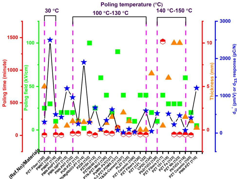
Fig. 9 Dependence of the  $d_{33}$  or  $d_{33}^*$  response of lead-based materials with poling conditions in Table 1.
