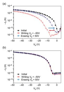
Fig. 5 Transfer characteristics of OFET memory devices fabricated using (a) TIPS-P/CuSP blend films and (b) TIPS-P/PS4 blend films monitored at
