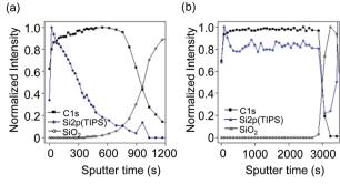
Fig. 4 XPS depth profiles of a TIPS-P/CuSP blend films coated from (a) ODCB and (b) CHCl<sub>3</sub> solutions on a Si substrate.
