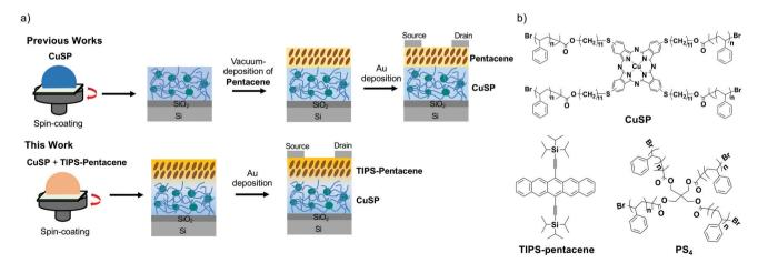
Fig. 1 (a) Schematic representation of the fabrication of OFET memory devices. (b) Chemical structures of TIPS-pentacene and polymer dielectrics of CuSP and PS<sub>4</sub>.
