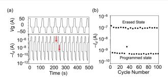
Fig. 6 WRER test (a) and endurance characteristics (b) of the OFET memory device with TIPS-pentacene/CuSP blend films.
