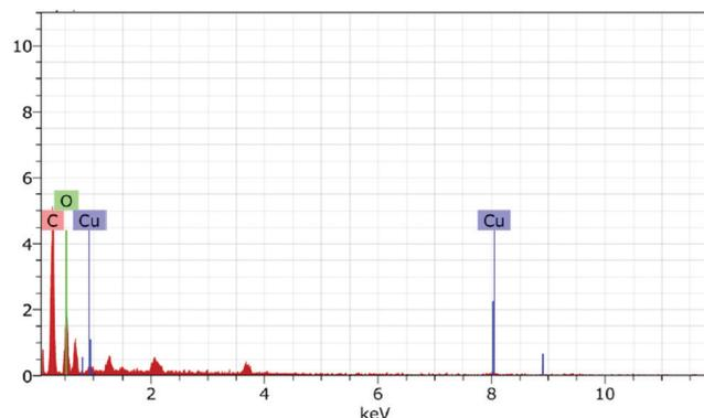
Fig. 4 EDX analysis of the biogenic CuO/rGO nanocomposite.
