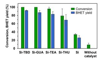
Fig. 3 The catalytic activities of different catalysts in PET glycolysis. Reaction conditions: 190 °C, 10 mol% (or 40 wt% in the case of Si) catalyst (if used), EG: PET ratio of 16, 2 h. BHET yield was determined by HPI C
