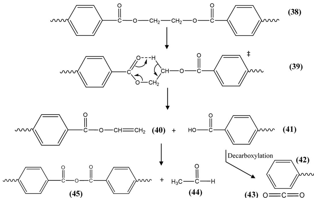
**Scheme 5** Fundamental reactions for the thermal decomposition of PET. The symbol ‡ indicates a transition state. Arabic numerals indicate chemical species and intermediates formed during the pyrolysis of PET.
