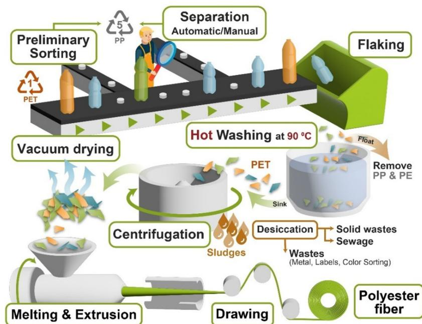
Fig. 14 A generalized process flow diagram for a recycling of PET bottles.<sup>150</sup>
