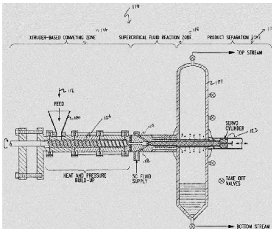
Fig. 23 Example of a continuous tubular reactor design for hydrothermal liquefaction of plastics (extracted from the US patent US 8980143B2).<sup>554</sup>
