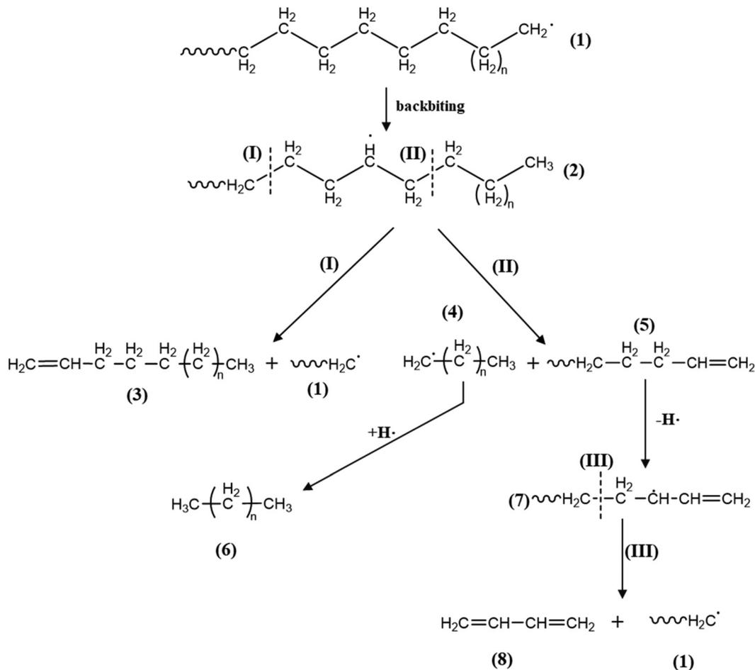
**Scheme 1** Fundamental reactions for the thermal decomposition of PE leading to alkanes (6), alkenes (5) and alkadienes (8). Arabic numerals indicate chemical species that form during the pyrolysis of PE, while Roman numerals indicate the occurrence and position of the scission of chemical bond.
