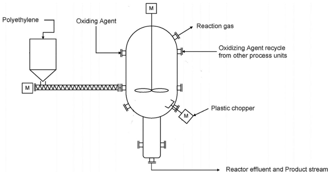
Fig. 42 The scheme of the ATOD reactor. (Extracted from the US patent US20220119616A1).<sup>902</sup>
