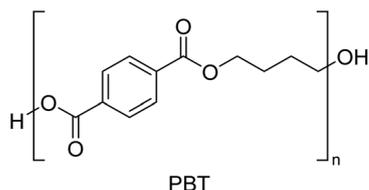
Fig. 39 Chemical structure of PBT.
