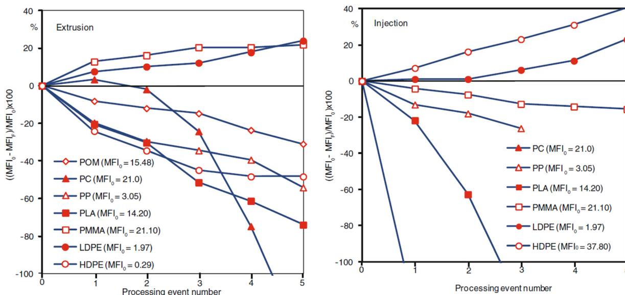
Fig. 12 Change in MFI as a function of number of processing events for extrusion (left) and injection molding (right). MFI<sub>0</sub> and MFI<sub>F</sub> are the MFI prior to any processing event and the MFI after the total processing events, respectively. Published from ref. 32 with permission from Carl Hanser Verlag, Munich, copyright 2012.
