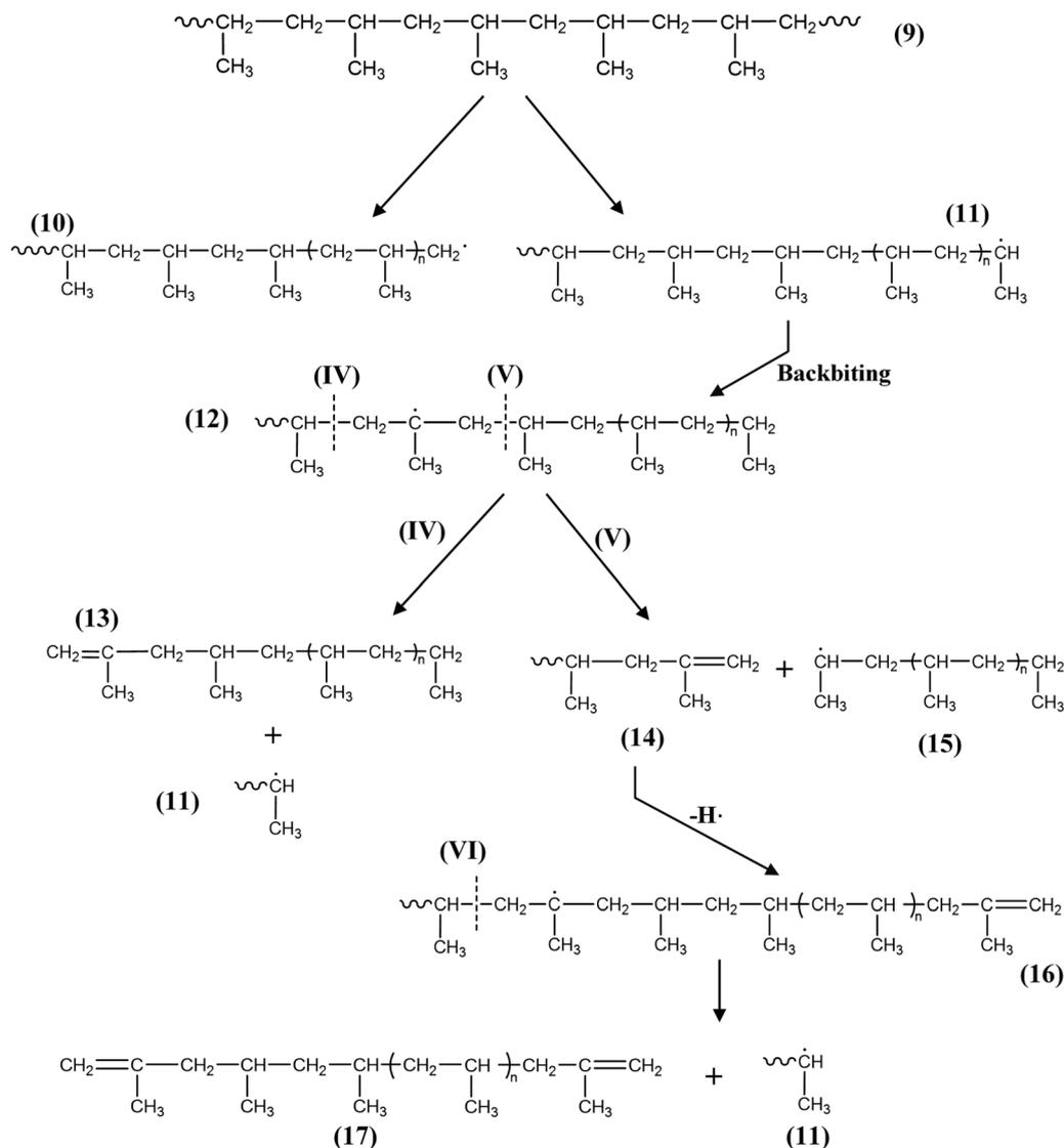
**Scheme 2** Fundamental reactions for the thermal decomposition of PP leading to alkenes and alkadienes. Arabic numerals indicate chemical species that form during the pyrolysis of PE, while Roman numerals indicate the occurrence and position of the scission of a chemical bond.
