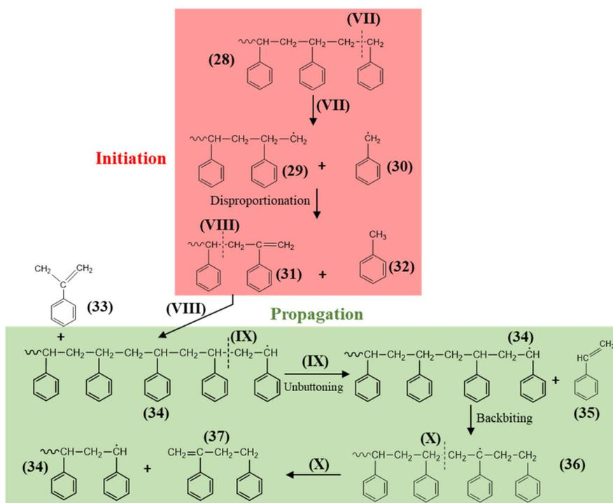
**Scheme 4** Fundamental reactions for the thermal decomposition of PS leading to different products. Arabic numerals indicate chemical species, while Roman numerals indicate the occurrence and position of the scission of a chemical bond.
