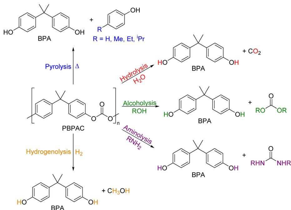
Fig. 38 Methods for the chemical depolymerization of PBPAC and their primary monomeric products.
