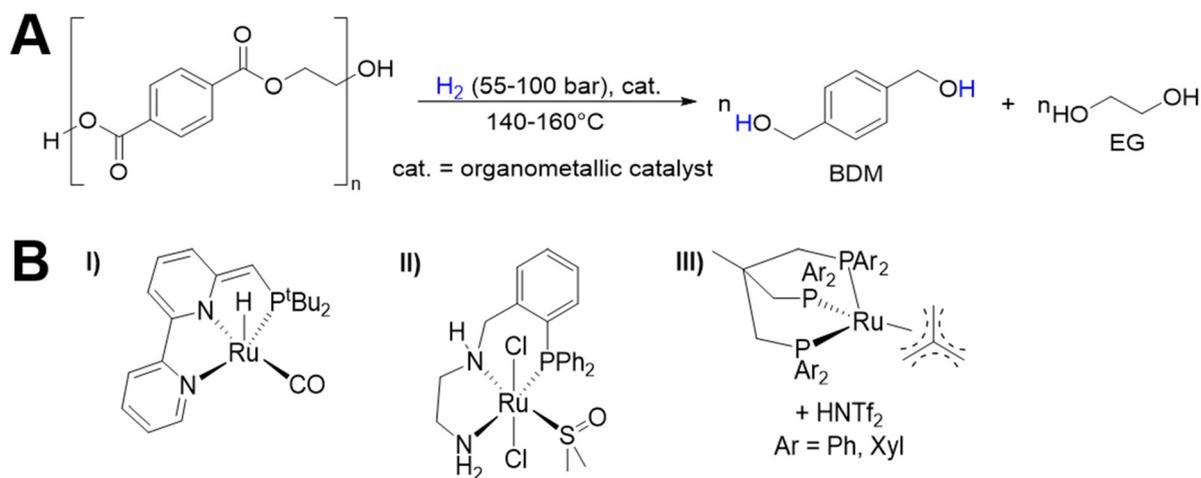
Fig. 36 (A) Typical reaction conditions and products for PET hydrogenolysis and (B) organometallic catalysts used for PET hydrogenolysis by (I) Krall *et al.*, (II) Fuentes *et al.*, and (III) Westhues *et al.*
