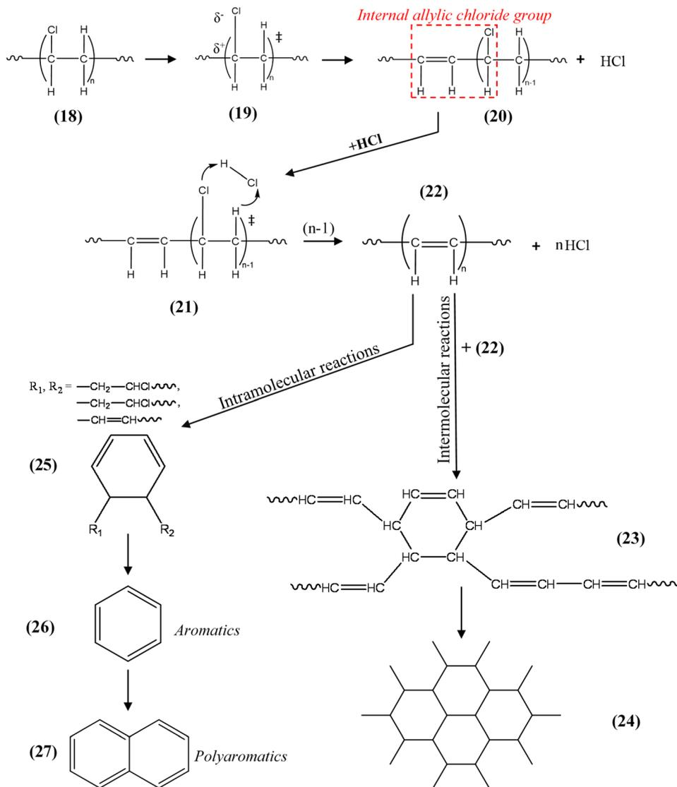
**Scheme 3** Fundamental reactions for the thermal decomposition of PVC leading to different products. The symbol  $\ddagger$  indicates a transition state. Arabic numerals indicate chemical species and intermediates that form during the thermal degradation of PVC.
