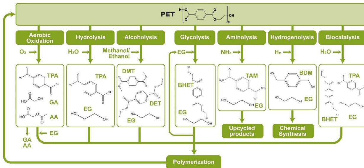
**Fig. 28** Strategies for PET chemical recycling discussed in this section, and their most common products. (TPA = terephthalic acid, EG = ethylene glycol, DMT = dimethylterephthalate, DET = diethylterephthalate, BHET = bis-2-hydroxyethylterephthalate, BDM = benzenedimethanol, MHET = mono-2-hydroxyethylterephthalate.)
