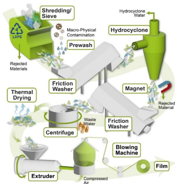
Fig. 15 Mechanical recycling process of polyethylene plastic film at an industrial plant.<sup>175</sup>
