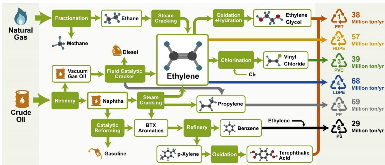
Fig. 3 Supply chain of the manufacture of #1–#6 plastics and their volume of production in 2019.<sup>19</sup>
