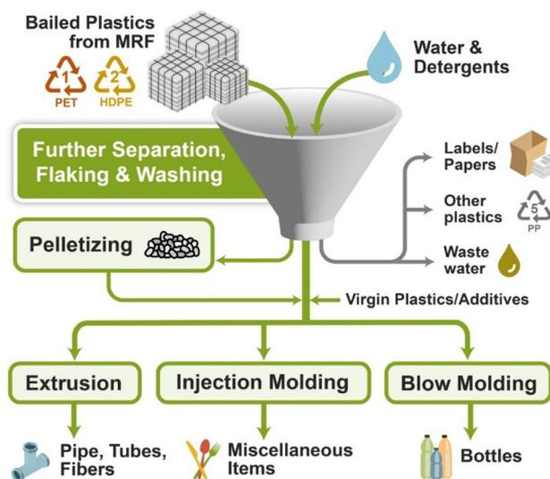
Fig. 13 Various approaches for mechanical recycling of PSW (plastic solid waste).<sup>136</sup>
