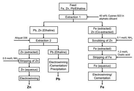
Fig. 16 Proposed flowsheet for the separation and recovery of Fe(III), Pb(II) and Zn(III) a mimicked jarosite waste stream. Reprint with permission from ref. 216, Copyright © 2020, Royal Society of Chemistry
