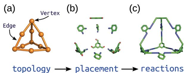
Fig. 4 Schematic of the construction process of an organic cage in *stk* starting from a (a) topology graph of vertices connected by edges. The supplied building blocks are (b) placed and aligned on the topology, and then (c) “reactions” are performed between them. Reprinted from ref. 95, with the permission of AIP Publishing.
