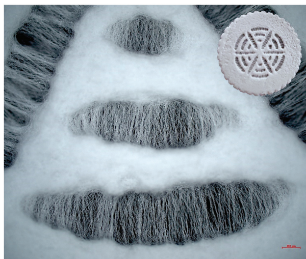
Fig. 4 Light microscopy image of radially and circumferentially oriented fibers in TM-sized membrane (scale bar 200 \mu\text{m} ) and whole membrane design ( \varnothing 10 mm, top-right corner).
