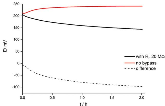
**Fig. 6** Dependence of open circuit potential on time for a potassium-selective ISE, non-bypassed (red line) and bypassed (black line) by zinc wire and resistor  $R_b = 20 \text{ M}\Omega$ . Dashed line: difference of potentials in the presence and absence of bypass.
