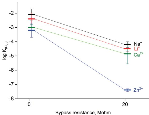
**Fig. 5** Effect of applied bypass resistance on the selectivity of potassium-selective ISE, mean value of logarithm of selectivity coefficient  $\pm$  SD is shown, the value presented was determined for activity range from  $10^{-3}$  to 0.1 M using experimental slopes.
