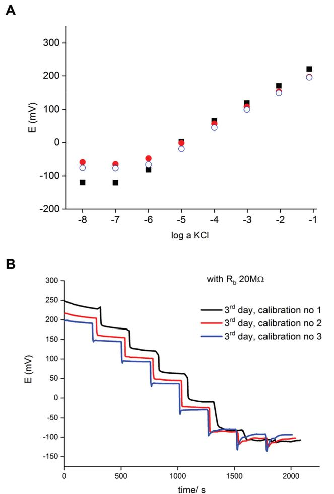
**Fig. 4** (A) Selected potentiometric calibration plots for potassium-selective ISE, bypassed by zinc wire and resistor  $R_b = 20$  M $\Omega$ , third calibration for each consecutive day is presented: (■) 1st day, (●) 2nd day (○) 3rd day. (B) Time traces for the sequential calibrations of the 3rd day.
