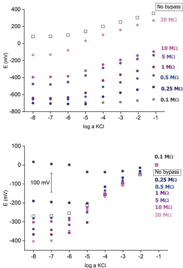
Fig. 2 Potentiometric calibration plots for  $\text{K}^+$ -selective ISEs, non-bypassed or bypassed by zinc wire and resistor  $R_b$ . Bottom panel: experimental points were shifted to common value for  $\log a \text{ KCl} = -1$ .
