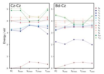
Fig. 5 Energy profiles for singlet and triplet states, including the  $Cz^-Cz^+$ and  $Cz^{-}Bd^{+}$  charge transfer states ( $S_{CT}$  and  $T_{CT}$ ) computed at the critical points for dimer A embedded in the crystal environment using the OEC model
