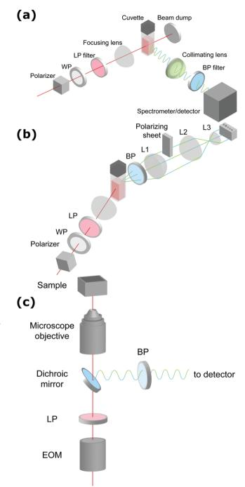
Fig. 1 Schematic representation of setups measuring (a) hyper-Rayleigh scattering, (b) angle-dependent second harmonic scattering through Fourier imaging (ref. 52), (c) polarimetric NLO microscopy (ref. 43). WP = wave-plate, LP = long pass filter, BP = band pass filter, L = lens, EOM = electro-optic modulator. The fundamental beam is depicted in red. the second and third harmonic light in green and blue respectively.
