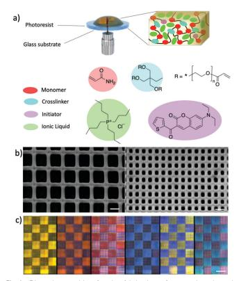
Fig. 1 Direct laser writing for the fabrication of responsive photonic structures. (a) Schematic of the direct laser writing process and photoresist composition; all structures were fabricated in the oil immersion configuration; SEM images (b) and angle-dependent optical microscopy images (c) of periodic photonic structures obtained through alternate fabrication of two types of square arrays, creating a checkerboard pattern. Scale bar represents 2.0 μm in (b) and 200 μm in (c).
