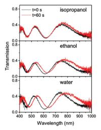
Fig. 3 Transmission spectra of the photonic structures of designed height  $h=3.5~\mu m$  with film, before (black) and after 1 min in the presence of solvent vapours (isopropanol – top; ethanol – middle and water – bottom) where the gas vapours were transported using dry air at a flow rate of 1 L min $^{-1}$ .
