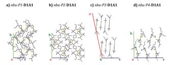
Fig. 5 Crystal structures (supercell) of nbu-Pn-D1A1 polymorphs as obtained in the current work, namely (a) nbu-P1- (chloroform, XRD at room temperature), (b) nbu-P2- (chloroform, XRD at 100 K), (c) nbu-P3-D1A1 (mesitylene, XRD at 100K); (d) nbu-P4-D1A1 as reported in ref. 28.
