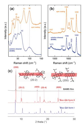
Fig. 6 (a) Lattice phonon and (b) intramolecular Raman spectra of spin cast and BAMS <sup>t</sup>Boc-QA films; (c) diffraction patterns of BAMS films and the two <sup>t</sup>Boc-QA polymorphs. Inset: Orientation of the two <sup>t</sup>Boc-QA molecules with respect of the (20-2) and (200) Miller planes in form II. H<sub>CH</sub> atoms omitted for clarity
