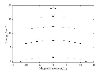
**Fig. 7** Calculated low-lying spin-orbit manifolds of states arising from the magnetic interaction between the ground multiplet S = 5/2 of the Fe<sup>III</sup> ion and the ground term <sup>8</sup>S of the Gd<sup>III</sup> ion in the [Fe<sup>III</sup>Gd<sup>III</sup>] complex. The components of each doublet (black lines) are placed on the diagram according to their magnetic moment projection on the main magnetic axis of the ground doublet (with energy zero).
