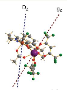
Fig. 9 Calculated molecular fragment of the [Fe<sup>III</sup>Tb<sup>III</sup>] complex (legend: Tb-indigo, Fe-brown, C-grey, N-blue, O-red, H-light grey). The dashed lines indicate the main anisotropy axis on Fe<sup>III</sup> ion (blue) and the main magnetic axis on Tb<sup>III</sup> ion (red).
