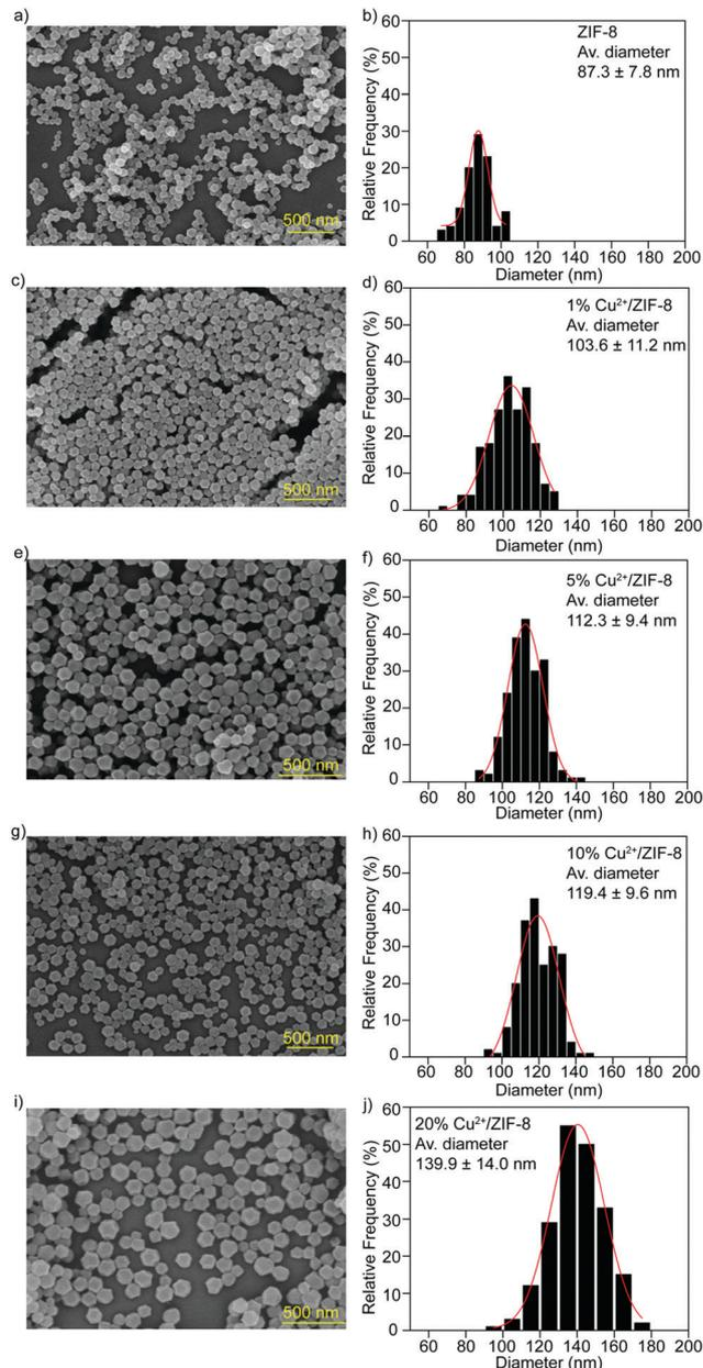
**Fig. 3** SEM images and size distributions of (a and b) ZIF-8, (c and d) 1% Cu<sup>2+</sup>/ZIF-8, (e and f) 5% Cu<sup>2+</sup>/ZIF-8, (g and h) 10% Cu<sup>2+</sup>/ZIF-8, and (i and j) 20% Cu<sup>2+</sup>/ZIF-8. Scale bars: 500 nm.
