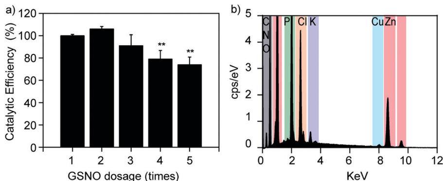
Fig. 6 (a) Catalytic efficiencies of 20% Cu<sup>2+</sup>/ZIF-8 particles (0.1 mg mL<sup>-1</sup>) after continuous addition of GSNO solutions (50 μM). Values represent mean ± standard deviation, *n* = 3. Statistical significance relative to the first dosage was calculated, \*\**p* < 0.01 (one-way ANOVA followed by Tukey *post hoc* test). (b) EDS spectrum of 20% Cu<sup>2+</sup>/ZIF-8 after reaction with GSNO.
