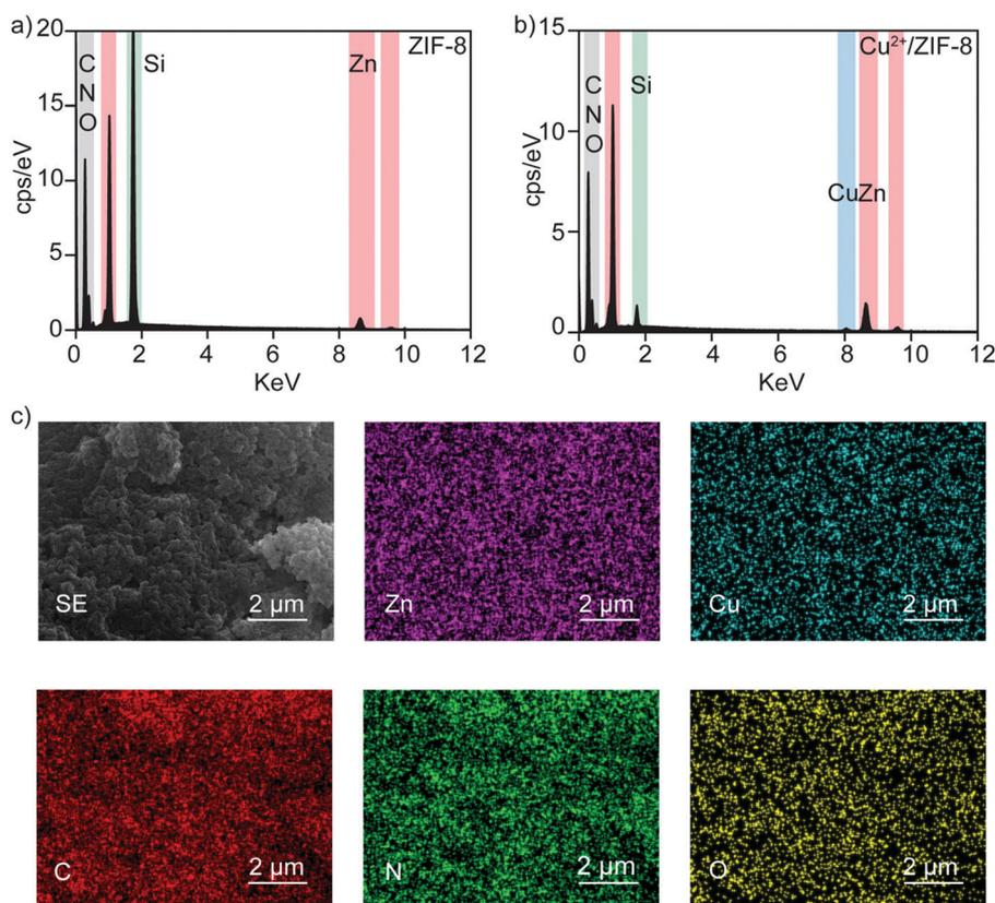
Fig. 2 EDS spectra of (a) ZIF-8 and (b) 20%  $\text{Cu}^{2+}$ /ZIF-8. (c) Elemental mapping of 20%  $\text{Cu}^{2+}$ /ZIF-8. Images shown are secondary electron (SE) image, elemental distribution of zinc (pink), copper (blue), carbon (red), nitrogen (green), and oxygen (yellow).
