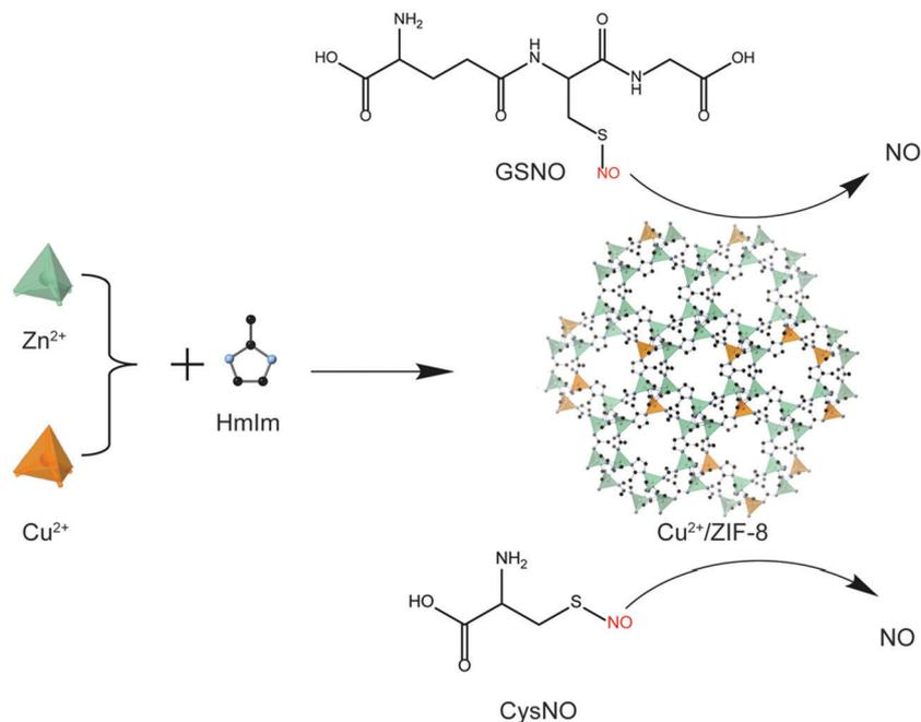
**Scheme 1** Schematic illustration of the synthesis of  $\text{Cu}^{2+}/\text{ZIF-8}$  which serves as a catalyst for *in situ* NO generation from NO prodrugs, S-nitrosoglutathione (GSNO) and S-nitrosocysteine (CysNO).
