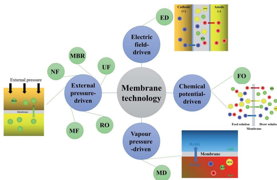
Fig. 1 Membrane technologies classified according to the driving force (MBR – membrane bioreactor, NF – nanofiltration, MF microfiltration, UF – ultrafiltration, RO – reverse osmosis, FO – forward osmosis, ED – electro dialysis, and MD – membrane distillation).
