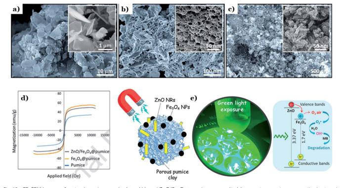
Fig. 19 FE-SEM images of: natural pumice powder (a and b), and  $ZnO/Fe_3O_4$ @pumice composite (c); room temperature magnetic-hysteresis (M-H) curves of the natural pumice,  $Fe_3O_4$ @pumice, and  $ZnO/Fe_3O_4$ @pumice composite (d); schematic of synergistic photocatalytic process, executed by  $ZnO/Fe_3O_4$ @pumice composite and green light irradiation (e). This figure has been reproduced (adapted) from ref. 127 with permission from Elsevier, copyright 2020.
