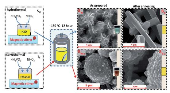
Fig. 6 Synthetic routes of the hydrothermal and solvothermal process for fabrication of  $V_2O_5$  nanorods and 3D (micro/nano)  $V_2O_5$  spheres. This figure has been reproduced from ref. 95 with permission from Springer, copyright 2019.
