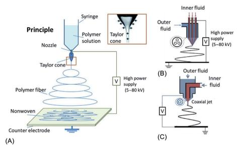
Fig. 10 Diagram illustration of the development of electrospinning technique: (A) principles; (B) three channel; and (C) one channel as inner fluids. This figure has been reproduced from ref. 111 with permission from Elsevier, copyright 2019.
