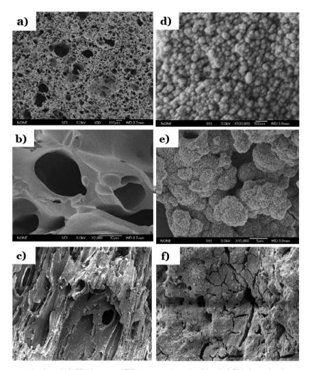
Fig. 18 SEM images of pure pumice (a and b); SEM images of  $TiO_2$ -mounted pumice (d and e). This figure has been reproduced (adapted) from ref. 126 with permission from Elsevier, copyright 2004. Micrographs of a pellet of: bare pumice (c), and pumice stone impregnated with  $TiO_2$ -P25 (f). This figure has been reproduced (adapted) from ref. 65 with permission from Elsevier, copyright 2003.
