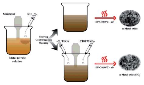
Fig. 8 Synthetic pathway of the coprecipitation process to fabricate nano-metal oxides (NiO, FeO and CoO) and nano-metal oxide/silicates. This figure has been reproduced from ref. 101 with permission from Elsevier, copyright 2015.
