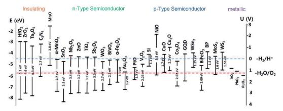
Fig. 4 Band-gap energies (eV) and energy levels of conduction band ( $E_{CB}$ ) and valence band ( $E_{VB}$ ) of semiconductors. This figure has been reproduced from ref. 57 with permission from Springer, copyright 2018.
