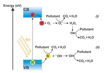
Fig. 3 Diagram illustration of photocatalytic reactions  $(h\nu \geq E_g)$ . Oxidation—reduction reactions of electron donors/acceptors occurred in CB (i) and VB (ii). This figure has been reproduced from ref. 45 with permission from Elsevier, copyright 2018.
