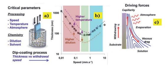
Fig. 7 Correlation between the thickness of film and speed of dip coating: (a)-dip-coating method and critical parameters; (b) correlation between the speed of coating and film thickness *versus* the dilution and temperature. (c) Correlation between the thickness of film and evaporation rate. This figure has been reproduced from ref. 99 with permission from RSC, copyright 2011.
