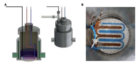
Fig. 12 Pressure vessel rig used for creation of surface electrostatics nanobubbles. (A) Cross section of the pressure vessel that include the gas supplier, distribution terminal the pressure cell and the temperature regulation jacket. (B) DC current supply set up *via* sheath covered wires in a 3 dimensional printed plastic.<sup>128</sup>
