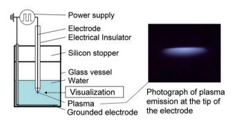
Fig. 18 Schematic of the experimental setup to form bulk nanobubbles *via* plasma generation in a specific volume of water. The plasma forms between the electrode tip placed in the water and the grounded electrode after turning on the high-voltage power supply.<sup>137</sup>
