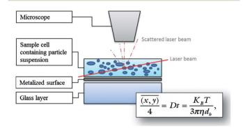
Fig. 7 Diagram illustrating the principle of NTA measurements using the Stokes–Einstein equation. Particles are illuminated by a laser light and movements of the particles are recorded through the scattered light *via* a CCD by a microscope. The software tracks the Brownian motion of each particle by determining the diffusion coefficient, and then calculates the size as the mean square of the particle path using the Stokes–Einstein equation.<sup>99</sup>
