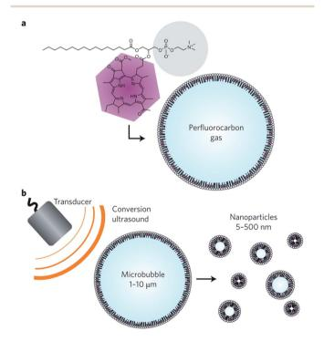
Fig. 16 Bulk nanobubbles generation *via* fragmentation of microbubbles. (a) A microbubble consists of bacteriochlorophyll–lipid and perfluorocarbon gas. (b) Production of bulk nanobubbles through applying low-frequency ultrasound to the bacteriochlorophyll–lipid shell microbubbles.<sup>132</sup>
