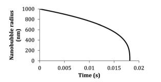
Fig. 1 Lifetime of a bubble smaller than 1000 nm predicted by the theory of Epstein and Plesset. The graph depicts the calculated radius of a nitrogen-filled bubble in a nitrogen saturated solution *versus* time ( $T=300~\rm K,~\gamma=0.072~\rm J~m^{-2},~D=2.0\times10^{-9}~m^2~s^{-1},~C_{sat}=0.6379~\rm mol~m^{-3},~\rho_{1~atm}=40.6921~\rm mol~m^{-3})$ , 8.9
