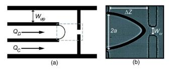
Fig. 22 Microbubble production by flow focusing. (a) A schematic drawing, and (b) microscopic image of flow focusing geometries. In (a),  $Q_{D_i}$ ,  $Q_{C_i}$  and  $W_{UD}$  represent the gas flow rate, liquid flow rate, and distance between the device wall and the gas channel, respectively. In (b), the orifice width, the gas flow channel width, and the junction-toorifice distance is shown by  $W_{\rm OR}$ , 2a, and  $\Delta Z$ , respectively. 154
