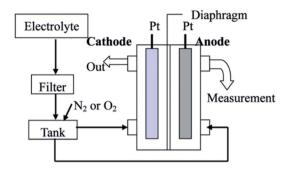
Fig. 17 Production of bulk nanobubbles through the electrolysis technique. An electrolyte solution passes from a filter with 100 nm holes before being merged with gas ( $O_2$  or  $N_2$ ) in the tank. Then, the mixed solution with gas in the tank transports to the chamber where the electrodes are placed. The electric current passing from the electrode anode to the cathode electrode electrolyzes the water inside the chamber.<sup>134</sup>
