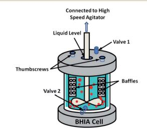
Fig. 9 Baffled high-intensity agitation (BHIA) cell used by Wu *et al.* to generate bulk nanobubbles. After introducing the solution into a baffled cell, the rotating impeller connected to a high-speed agitator creates hydrodynamic cavitation leading to the generation of bulk nanobubbles. Valves 1 and 2 are used to take samples for the characterization of the generated bulk nanobubbles. The thumbscrews are placed to tightly seal the cap cell to the cell body.<sup>118</sup>
