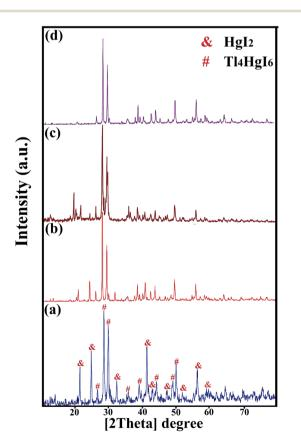
Fig. 2 XRD patterns obtained from  $Tl_4Hgl_6/Hgl_2$  nanocomposite in different surfactant; (a) SDS, (b) NaHSal, (c) EDTA, and (d) PVP.
