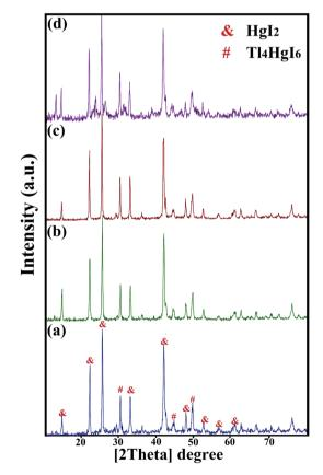
Fig. 3 XRD patterns obtained from  $Tl_4Hgl_6/Hgl_2$  nanocomposite in a different time and power of sonication; (a) 20 minutes, 40 watt, (b) 20 minutes, 80 watt, (c) 10 minutes, 60 watt, and (d) 30 minutes, 60 watt.
