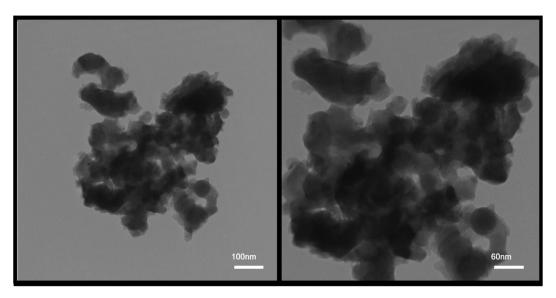
Fig. 7 TEM images from the sample prepared in the presence of PVP as the optimal sample (sample no. 8).
