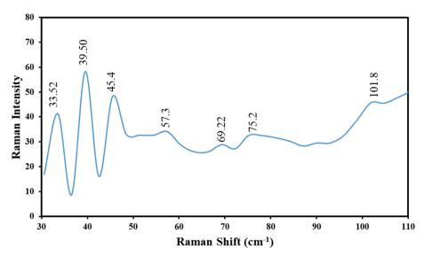
Fig. 8 Raman spectrum of Tl<sub>4</sub>Hgl<sub>6</sub>/Hgl<sub>2</sub> nanocomposite (sample no. 8) at ambient temperature (25 °C).
