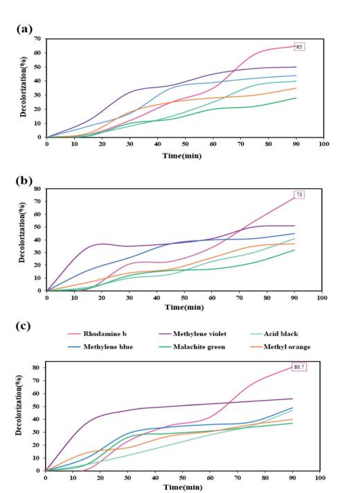
Fig. 12 Photocatalysis test results for six dyes in the presence of different amounts of  $Tl_4Hgl_6/Hgl_2$  nanocomposite (a) 0.03 gr, (b) 0.05 gr, and (c) 0.07 gr.
