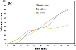
Fig. 13 (a) Evaluation of the stability of photocatalytic activity of  $Tl_4Hgl_6/Hgl_2$  nanocomposite on rhodamine b decolorization, (b) photocatalytic activity of  $Tl_4Hgl_6/Hgl_2$  nanocomposite in the presence of scavengers.
