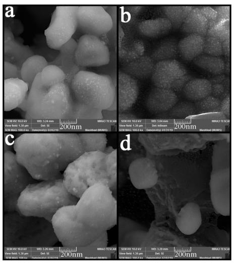
Fig. 4 SEM images of synthesized nanocomposites using different ratios of Tl to Hgl<sub>2</sub> precursors; (a) 1:1, (b) 2:1, (c) 3:1, and (d) 1:2.
