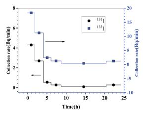
Fig. 4 Collection rates of <sup>131</sup>I and <sup>133</sup>I on the Ni foils.
