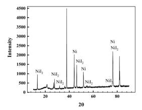
Fig. 5 XRD pattern of the deposits on the Ni foil.
