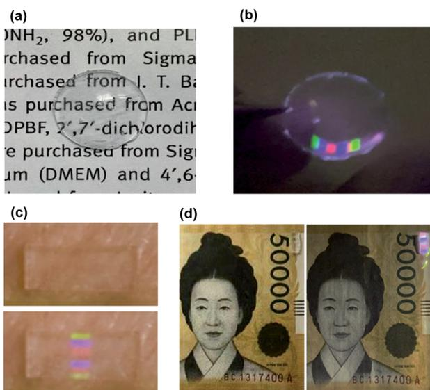
Fig. 7 Photoimages of UCNPs-barcode patterned contact lens on letters under (a) indoor-room light and (b) 980 nm NIR light ( $500 \text{ mW cm}^{-2}$ ) in the dark field. Photoimages of UCNPs barcode patch on (c) porcine skin and (d) paper currency under indoor-room light and 980 nm NIR light.
