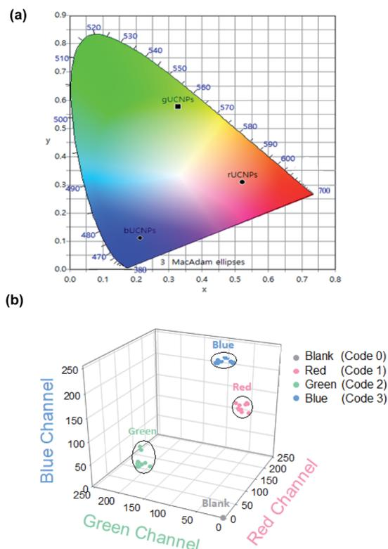
**Fig. 4** (a) CIE color coordinates of rUCNP, gUCNP and bUCNP-PDMS composites. (b) The RGB values plot of red (rUCNPs-PDMS), green (gUCNPs-PDMS) and blue (bUCNPs-PDMS) in 3D RGB channel map and the assigning codes ( $n = 10$ ).
