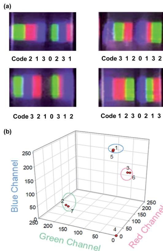
Fig. 6 (a) Photoimages of 7-digit barcode patches under 980 nm light ( $500 \text{ mW cm}^{-2}$ ) and the assigned codes. (b) The decoding plot for the assigned code of '3210312' in the 3D RGB channel map.
