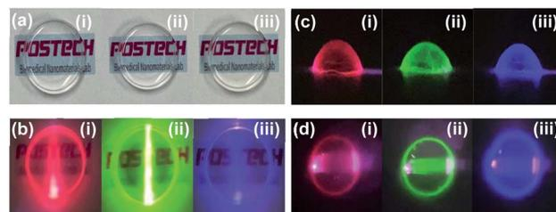
**Fig. 3** (a) The photoimages and (b) the upconversion emission images under 980 nm light ( $500 \text{ mW cm}^{-2}$ ) of (i) rUCNPs-PDMS, (ii) gUCNPs-PDMS and (iii) bUCNPs-PDMS composites. The photoimages of UCNP embedded color lenses: (c) side view and (d) top view under 980 nm light ( $500 \text{ mW cm}^{-2}$ ).
