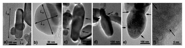
Fig. 1 TEM images of LiFePO<sub>4</sub> powders in the samples: (a) no. 1, (b) no. 2. The measured width  $L_s$  and length  $L_b$  of the particle are shown with arrows. (c)–(e), (f) – fused and mosaic particles, respectively. The arrows show the boundaries between the blocks.
