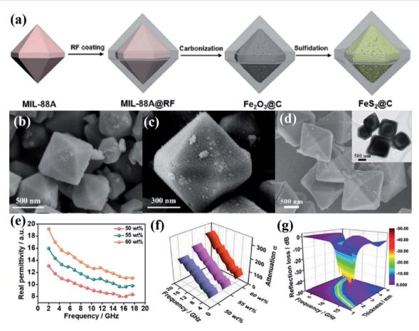
Fig. 9 The schematic formation process of  $FeS_2/C$  composites (a), SEM images of Fe-MOF (b),  $Fe_3O_4/C$  (c), SEM and TEM images of  $FeS_2/C$  (d), the real permittivity (e), attenuation constant (f) and the RL of  $FeS_2/C$  composites (g). This figure has been reproduced from ref. 16 with permission from Nano Letters, Copyright 2020.
