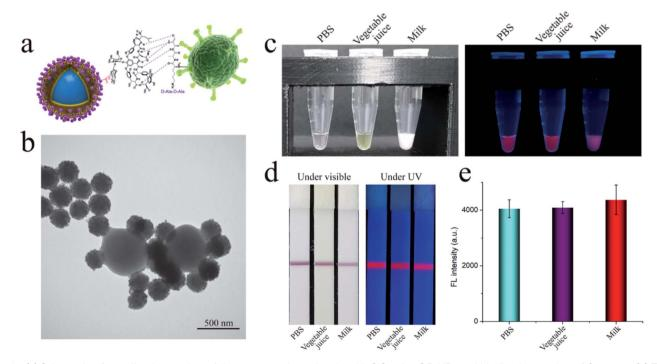
Fig. 2 (a) Schematic of coupling interaction of the vancomycin molecule with  $SiO_2$ -Au-QD NPs and binding interaction of S. aureus. (b) TEM image of formed Van-nanotags-S. aureus complexes. (c) Photographs and fluorescence images of Van-nanotags in different samples (PBS, vegetable juice, and milk). Photographs (d) and corresponding fluorescence intensity (e) of SiO<sub>2</sub>-Au-QD-Van based LFA strips in PBS, vegetable juice, and milk.
