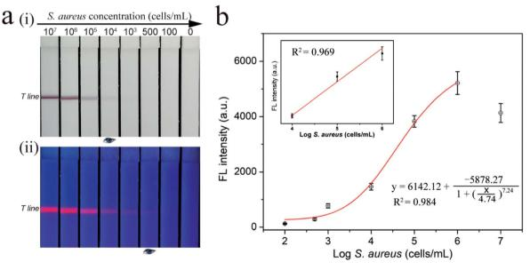
Fig. 3 Detection performance of SiO<sub>2</sub>-Au-QD-Van based LFA strip in milk sample. (a) Photographs (i) and fluorescence pictures (ii) of SiO<sub>2</sub>-Au-QD-Van-based LFA strip for different concentrations ( $10^7$  to 0 cells mL $^{-1}$ ) of S. aureus in milk samples. (b) Corresponding calibration curves for S. aureus. Inset in (b) is the linear part of the calibration curve. Error bars indicating the standard deviation of three independent tests.
