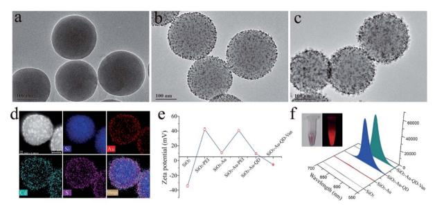
Fig. 1 Characterization of dual-signal SiO<sub>2</sub>-Au-QD nanotags. TEM images of (a) SiO<sub>2</sub> NPs, (b) SiO<sub>2</sub>-Au NPs, and (c) SiO<sub>2</sub>-Au-QD NPs. (d) EDS elemental mapping images of SiO<sub>2</sub>-Au-QD tags. Zeta potential results (e) and fluorescence emission spectra (f) of vancomycin-modified nanotags and their intermediate products. Inset images display the photographs of SiO<sub>2</sub>-Au-QD-Van tags under visible (left) and UV light (right).
