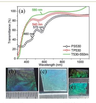
Fig. 5 UV-vis-NIR transmittance spectra of PS530 (black diamonds) (a), TP530 (red circles), T530-550im (green trace), and optical photos for samples TP530 supported on ITO (b) and silicon chips (d); T530-550im supported on ITO (c) and silicon chips (e).
