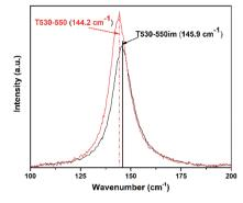
Fig. 3 Raman spectra of samples T530-550 and T530-550im illustrating the shift of the main  $E_{\alpha}$  peak from the presence of sulphur ions.
