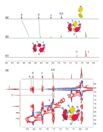
Fig. 1 Partial  $^{1}$ H NMR spectra (400 MHz, acetone- $d_{6}/D_{2}O = 1:1$ , room temperature) of (a)  $\mathbf{M}$  (1.00 mM), (b)  $\mathbf{H}'$  (1.00 mM) and  $\mathbf{M}$  (1.00 mM), and (c)  $\mathbf{H}'$  (1.00 mM). (d) Partial NOESY NMR spectrum (400 MHz, acetone- $d_6$ /  $D_2O = 1:1$ , room temperature) of  $\mathbf{H}' \supset \mathbf{M}$  (5.00 mM).
