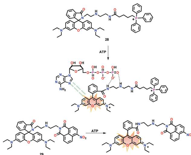
Fig. 13 Chemical drawings of chemosensors 28 and 29 and their proposed binding with ATP through  $\pi \cdots \pi$  interactions with the open conformation of the spirolactam ring. Adapted from ref. 57 and 58.
