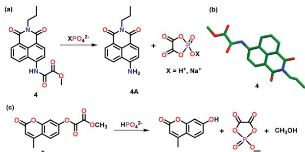
**Fig. 3** (a) Chemical drawing of chemosensor 4 and its proposed 'Turn-On' emission mechanism with  $XPO_4^{2-}$  ion ( $X = H^+$  or  $Na^+$ ). (b) Crystal structure of the chemosensor 4. (c) Chemical drawing of chemosensor 5 and its 'Turn-On' emission mechanism with  $HPO_4^{2-}$  ions. Adapted from ref. 43 and 44.
