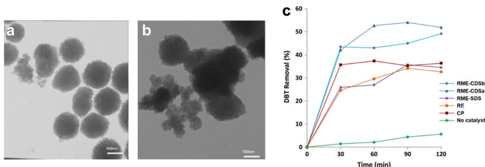
Fig. 11 TEM images of CsPW synthesized *via* (a) reverse microemulsion (RME) method and (b) co-precipitation (CP) method. (c) DBT removal with TBHP at 60 °C over various CsPW created by CP, reversed emulsion (RE) method and RME with sodium dodecyl sulfate (SDS) or caesium dodecyl sulfate (CDS) as surfactant. Reprinted with permission.<sup>145</sup> Copyright 2020, Springer Nature.
