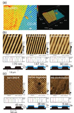
**Fig. 7** (a) Laser microscope images of the edge of the  $[(Ala)_{10}-PPG]_m$  nanofilm (300 nm thick) on a CD-R surface. (b) and (c) AFM images of bare and  $[(Ala)_{10}-PPG]_m$  nanofilms (150 nm and 300 nm thick)-coated CD-R (b) and DVD-R (c) surfaces and their corresponding height profiles.
