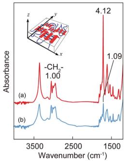
Fig. 6 (a) Transmission- and (b) reflection absorption-FTIR spectra of the  $[(Ala)_{10}-PPG]_m$  nanofilm (300 nm thickness) on a  $CaF_2$  plate and Au plate, respectively. The inset shows a schematic illustration of the orientation of β-sheet multiblocks in the nanofilm.
