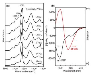
Fig. 2 (a) Transmission FTIR spectra of various  $[(peptide)_n - PPG]_m$  microfilms. (b) CD spectra of  $[(Ala)_8 - PPG]_m$  in HFIP (2 mg mL<sup>-1</sup>) and at the film state on a quartz plate.
