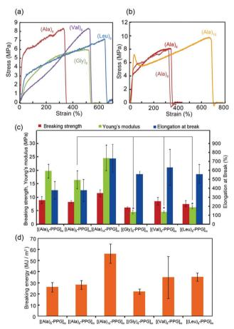
Fig. 3 Mechanical properties of  $[(peptide)_n - PPG]_m$  hybrid microfilms. (a and b) Representative stress-strain curves of various  $[(peptide)_n-PPG]_m$ films with different peptide sequences (a) and chain lengths (b). (c) Summary of tensile tests. Statistical analyses performed using Student's t-test. \*p < 0.01. (d) Comparison of breaking energy for [(peptide)<sub>n</sub>-PPG]<sub>m</sub> films. Error bars represent standard deviation
