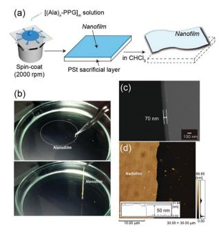
Fig. 5 (a) Preparation of the self-supporting  $[(Ala)_n - PPG]_m$  nanofilm *via* spin coating using a sacrificial under layer. (b) Photographs of the  $[(Ala)_n]$ PPG]<sub>m</sub> nanofilm in CHCl<sub>3</sub> (top) and that grasped using tweezers (bottom). (c) Cross-sectional SEM and (d) AFM images of the  $[(Ala)_8-PPG]_m$  nanofilm obtained from 0.5 wt% solution. The inset in (d) shows the height profile at the edge of the nanofilm
