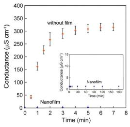
Fig. 8 Time courses of ion permeation (NaCl) through the  $[(Ala)_{10}-PPG]_m$ nanofilm (300 nm thickness). The inset shows the time course of electrical conductance over a long duration (180 min). Errors indicate standard deviation
