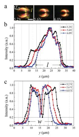
Fig. 3 Dependence of soliton size on voltages. (a) Polarizing optical micrographs of a soliton at different applied voltages at frequency f = 1 kHz. The yellow lines intersect the soliton along the x- and y-axes indicate the length (I) and width (w) of the soliton. Transmitted light intensity profiles of the soliton measured as a function of (b) x-coordinate and (c) y-coordinate along the yellow lines in (a) at varied voltages. f = 1 kHz, T = 34.0 °C, scale bar 10  $\mu$ m.
