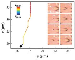
Fig. 9 Trajectory of a swallow-tail soliton nucleated from a microparticle. The color bar represents the elapsed time.  $t_{\rm Min}=0$  s,  $t_{\rm Max}=17.5$  s, time interval  $\Delta t=0.5$  s. Insets are time series of micrographs of the nucleation of a soliton at a micro-particle. U=7.6 V, f=10 Hz, T=33.5 °C, scale bar 10 μm, micro-particle diameter  $R_{\rm P}=1.5$  μm.
