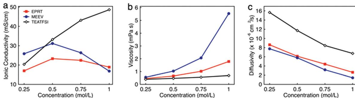
**Fig. 3** The ionic conductivity (a), viscosity (b), and diffusivity (c) of EPRT-TFSI, MEEV-(TFSI)<sub>2</sub>, and TEATFSI at 0.25, 0.50, 0.75, and 1.00 M in ACN. The uncertainties associated with measurements are reported in the Table S1 (ESI<sup>†</sup>), as the uncertainty bars are smaller than the symbol size on the graphs.
