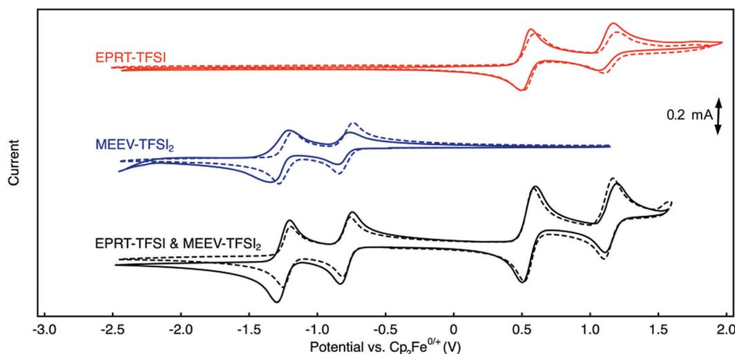
Fig. 4 Cyclic voltammograms of EPRT-TFSI (red, top traces), MEEV-(TFSI)<sub>2</sub> (blue, middle traces), and an equimolar combination of both EPRT-TFSI and MEEV-(TFSI)<sub>2</sub> (black, lower traces) at 10 mM in ACN with no supporting salts (solid-line) and in ACN with 0.5 M TEATFSI (dashed-line). CV experiments were performed at a scan rate of 100 mV s<sup>-1</sup>, and 100% iR correction was applied. All voltammograms are referenced to ferrocene/ferrocenium at 0 V.
