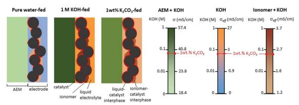
Fig. 3 Schematic illustration of a half cell with supplying pure water, 1 M KOH, or  $1 \text{ wt}\% \text{ K}_2\text{CO}_3 \text{ solution}$ . We estimated the conductivity of AEM from the high-frequency resistance of the cell using an HTMA-DAPP AEM as a function of KOH concentration at 50 °C.
