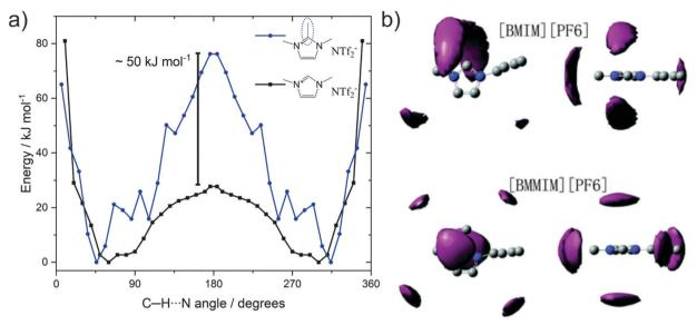
Fig. 20 (a) Energy as a function of the angle between C2 carbon, acidic hydrogen, and imide-N of the [NTf<sub>2</sub>].<sup>255</sup> (b) Spatial distribution function of [PF<sub>6</sub>] around  $[C_4C_1im]$  (top) and  $[C_4C_1C_1im]$  (bottom). Reproduced from ref. 257 with permission from the PCCP Owner Societies
