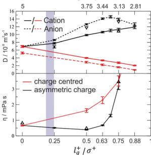
Fig. 16 Diffusion and viscosity as a function of charge separation. The blue shaded area indicates the  $l_a^+/\sigma^+$  range for the [C<sub>4</sub>C<sub>1</sub>im] cation. The charge centred systems where charge separation is achieved by decreasing the size are shown in red. Reprinted (adapted) from H. V. Spohr and G. N. Patey, J. Chem. Phys., 2009, 130, 104506, with the permission of AIP Publishing.217
