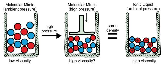
Fig. 2 The effect of Coulombic compactisation on the viscosity of ionic liquids can be investigated with molecular mimics, i.e. a targeted modification that replaces cations and anions with isostructural neutral molecules.
