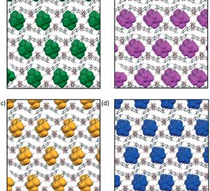
1 The isostructural solvates of 1 (1,10-phenanthronilium pamoate). (a) 1.DMF, (b) 1.DMA, (c) 1.DMSO and (d) 1.THF. The host ions are shown in stick representation, whilst the guest molecules are shown in spacefill representation with each guest in a different colour.
