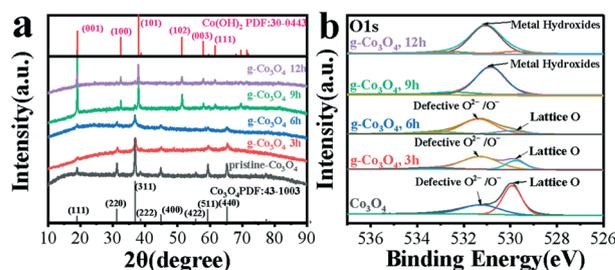
Fig. 3 (a) The XRD patterns and (b) O1s spectra of pristine  $\text{Co}_3\text{O}_4$  (black) and g- $\text{Co}_3\text{O}_4$  with different hydrothermal reaction times: (red) 3 h; (blue) 6 h; (green) 9 h and (purple) 12 h.
