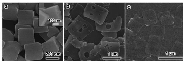
**Fig. 3** FESEM images of the ZIF-8 products at SDS concentrations of (a) 4, (b) 16 and (c) 91 mM, respectively. The inset is the cross-sectional FESEM image of the obtained ZIF-8 cubic crystals.
