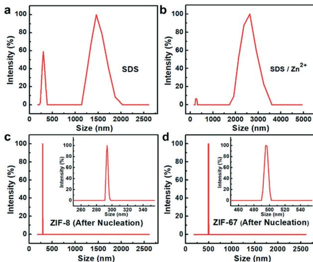
Fig. 5 DLS measurements of (a) the SDS aqueous solution and (b) the SDS and zinc ion mixture, and nucleus dispersions after adding ligands for (c) the ZIF-8 and (d) ZIF-67 reaction systems, respectively.
