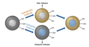
Scheme 1 Loading of an entirely porous core-shell nanoparticle consisting of a hydrophilic silica core and a hydrophobic organosilica shell. Hydrophobic (orange) and hydrophilic guest molecules (blue) are selectively adsorbed at different parts of the nanoparticles, leading to different release behaviors depending on the diffusion path length.
