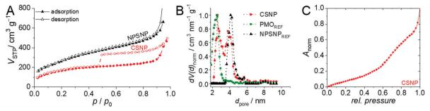
Fig. 2 Results of physisorption measurements. (A) Nitrogen physisorption isotherms for NPSNPs (black) and CSNPs (red). (B) Normalized pore size distributions; the pore size distributions of a pure PMO material (red) and a pure NPSNP material (black) are shown for reference; note that the CSNP sample shows two maxima which can be assigned to the NPSNP core and the PMO shell. (C) Normalized water adsorption isotherm of CSNPs at 25 °C with an increasing slope from a relative pressure of 0.6.
