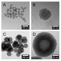
Fig. 3 TEM images of NPSNPs (A and B) and CSNPs (C and D). (A) Non-agglomerated spherical NPSNPs with a particle diameter of *ca.* 40 nm; (B) close-up revealing the porous nature. (C) Spherical CSNPs with a particle size of *ca.* 80 nm containing in most of cases only one core; (D) close-up revealing the core-shell character of the CSNPs; the shell has a thickness of *ca.* 20 nm.
