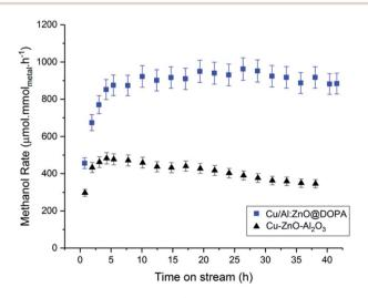
Fig. 6 Methanol rates of Cu/Al:ZnO@DOPA and commercial heterogeneous Cu-ZnO-Al<sub>2</sub>O<sub>3</sub>, over 40 h time-on-stream.
