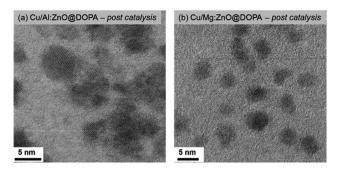
Fig. 5 BF-TEM images of the post-catalysis sample of (a) Cu/Al:ZnO@DOPA and (b) Cu/Mg:ZnO@DOPA.
