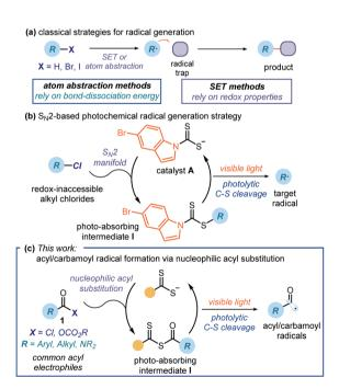
Fig. 1 (a) Traditional strategies for generating radicals require precursors with suitable bond-dissociation energies (BDE) or redox properties. (b) Our recently developed  $S_N2$ -based method uses a nucleophilic dithiocarbamate anion catalyst A to photochemically generate radicals based on the electrophilicity of substrates. (c) Presented photochemical generation of acyl and carbamoyl radicals based on a nucleophilic acyl substitution mechanism.
