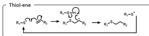
Fig. 12 Mechanism of thiol-ene catalytic reaction.
