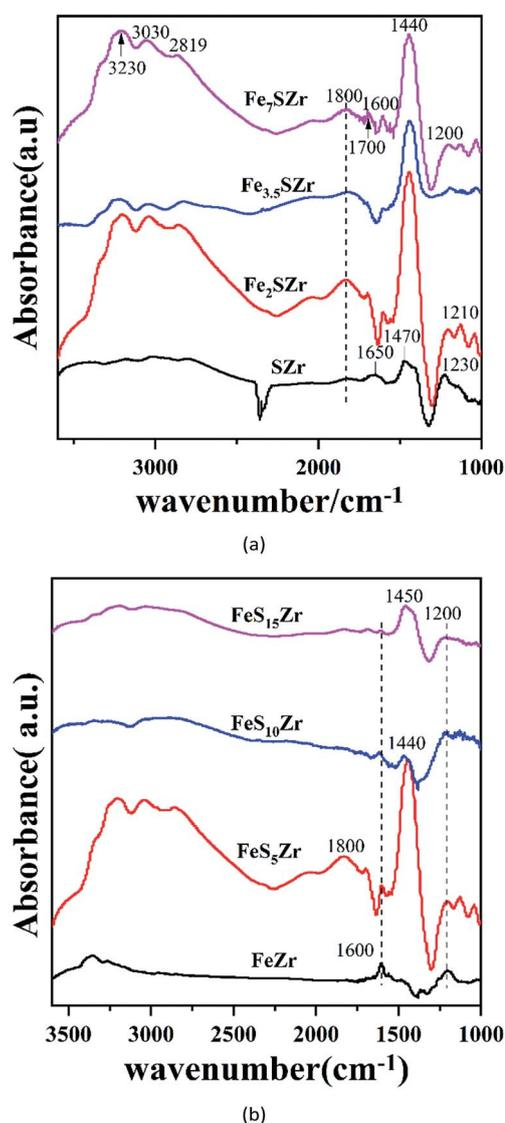
Fig. 7 Infrared spectra of a series of catalysts with the saturated adsorption of NH<sub>3</sub> at 30 °C and after purging with N<sub>2</sub>: (a) catalysts containing 5% SO<sub>4</sub><sup>2-</sup> and x% Fe<sup>3+</sup> (x = 0, 2, 3.5, 7) and (b) catalysts containing 3.5% Fe<sup>3+</sup> and y% SO<sub>4</sub><sup>2-</sup> (y = 0, 5, 10, 15).
